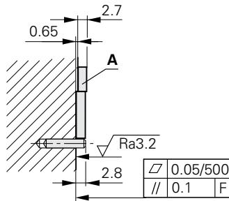
The mounting surface must be free of paint, dust, or grease.
