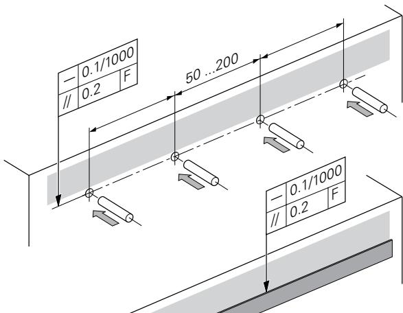
The scale with PRECIMET adhesive mounting film has to be attached at a temperature > 15 °C! Pay attention to the expiration date on the package! Peel off the protective film from the mounting film, protect the adhesive surface from contamination!
