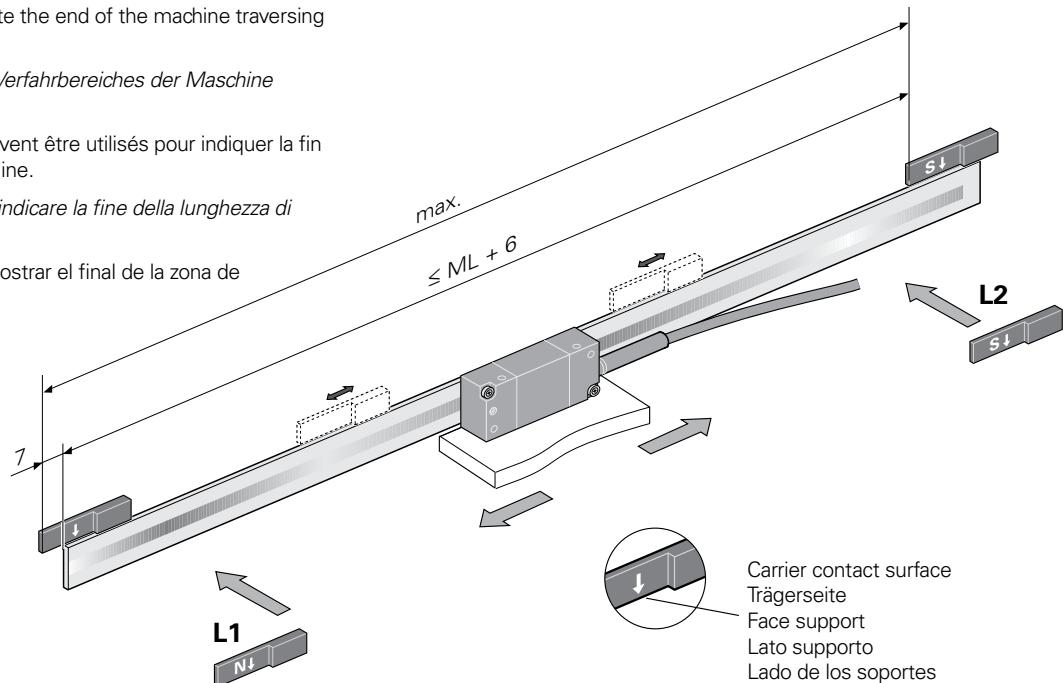
To display the switching point, use an adapter. To do this, move the scanning head to the desired position and insert the magnet.
