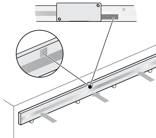
Use the roller to evenly press the scale against the mounting surface, starting from the middle.
