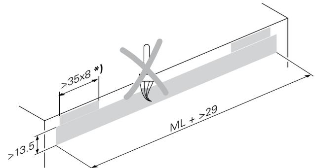
Mount the aligning rail.
