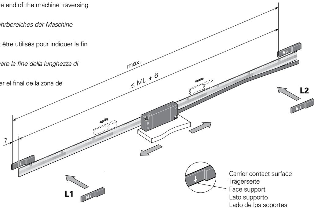
To display the switching point, use an adapter. To do this, move the scanning head to the desired position and insert the magnet.
