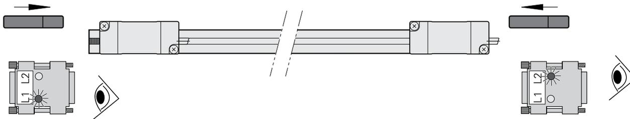
**Please note:** If the limit switches are configured as active high, the LED display is also inverted.
