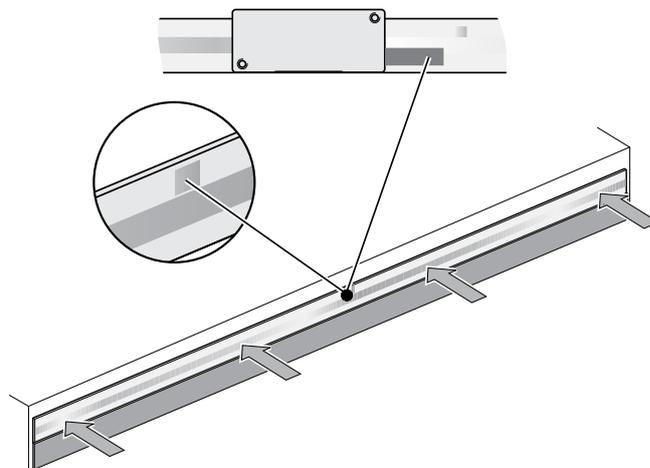
Starting from the middle, press the scale tape evenly onto the mounting surface using a roller.
