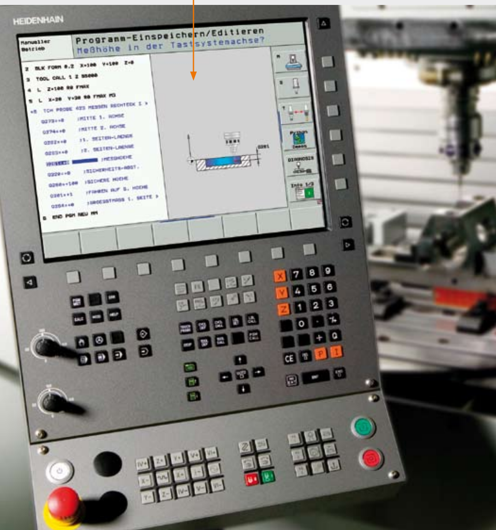
TNC cycle: Setting the datum for the aligned workpiece.
