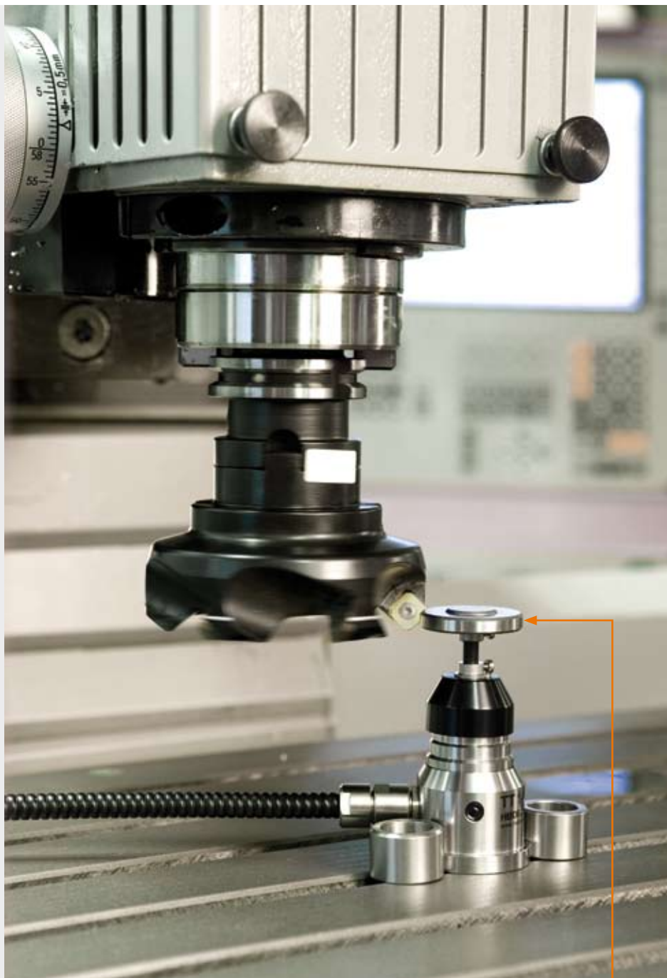
Wear-free and dependable tool measurement via disk-shaped TT 140 probing element
